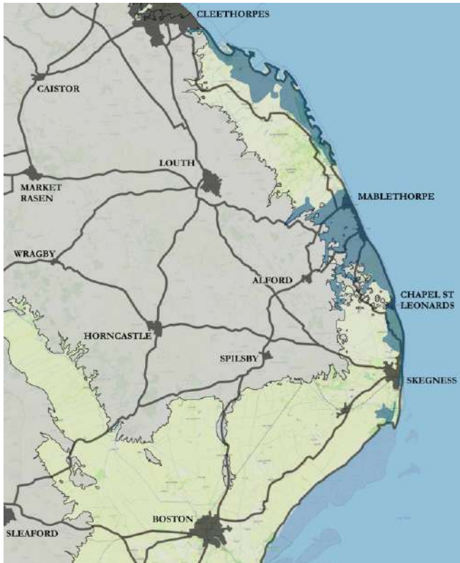
Figure 146: The extent of the sea flooding along the Lincolnshire coast in 1953, after Barnes and King, Robinson, and Steers (see fn. 686). Note, the flooding occurred mainly on the Outmarsh and was constrained north of Mablethorpe by the presence of saltern mounds, storm beaches and a substantial dune belt in this area (Underlying modern mapping © OpenStreetMap contributors, available under the Open Database Licence).
